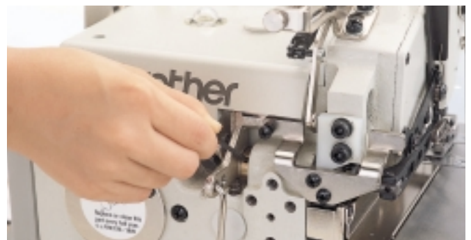
Adjusting upper feed vertical amount
