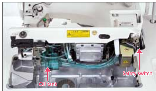
Designed with no oil pan (minute-quantity lubrication type)
